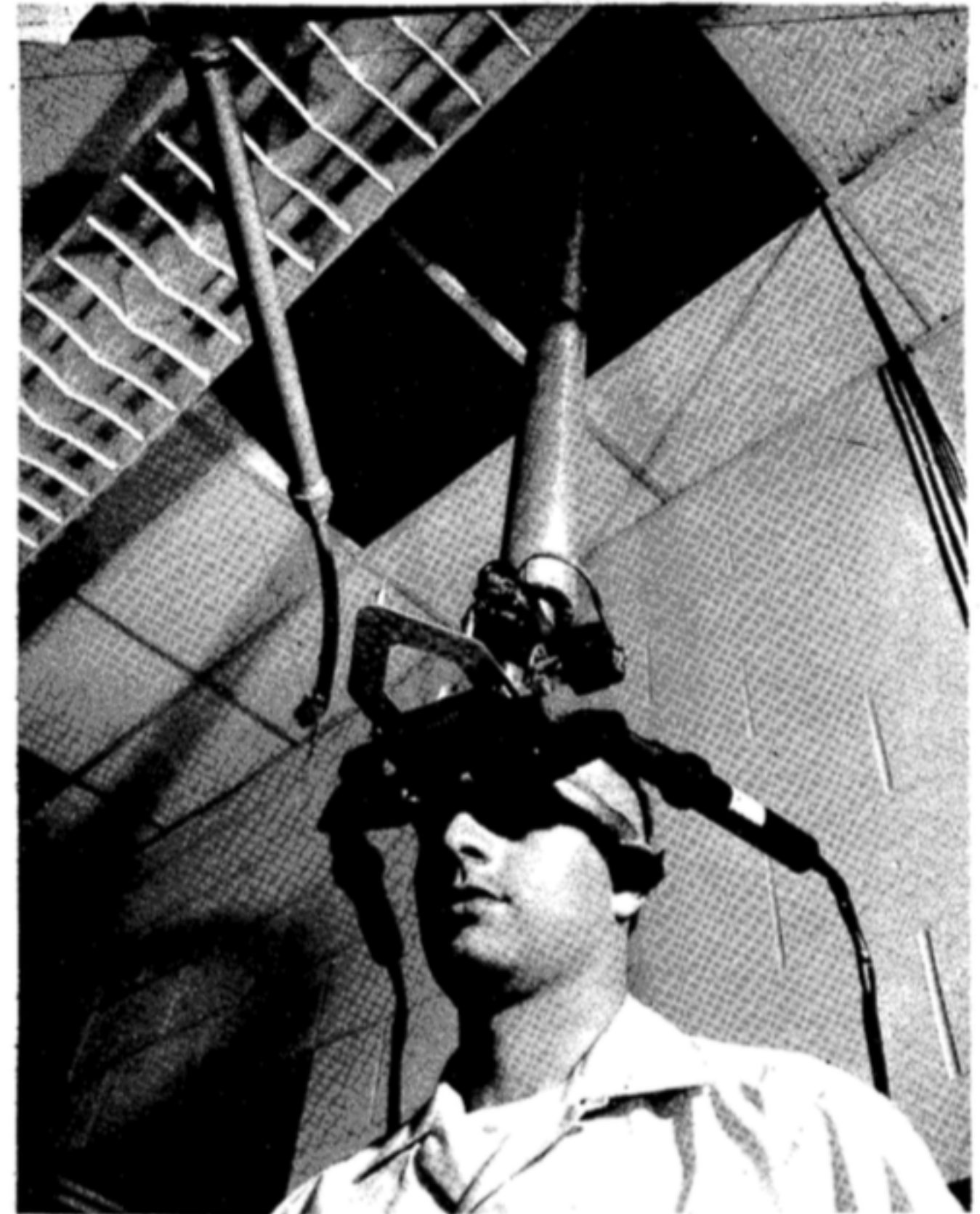
FIGURE 4—The ultrasonic head position sensor in use
