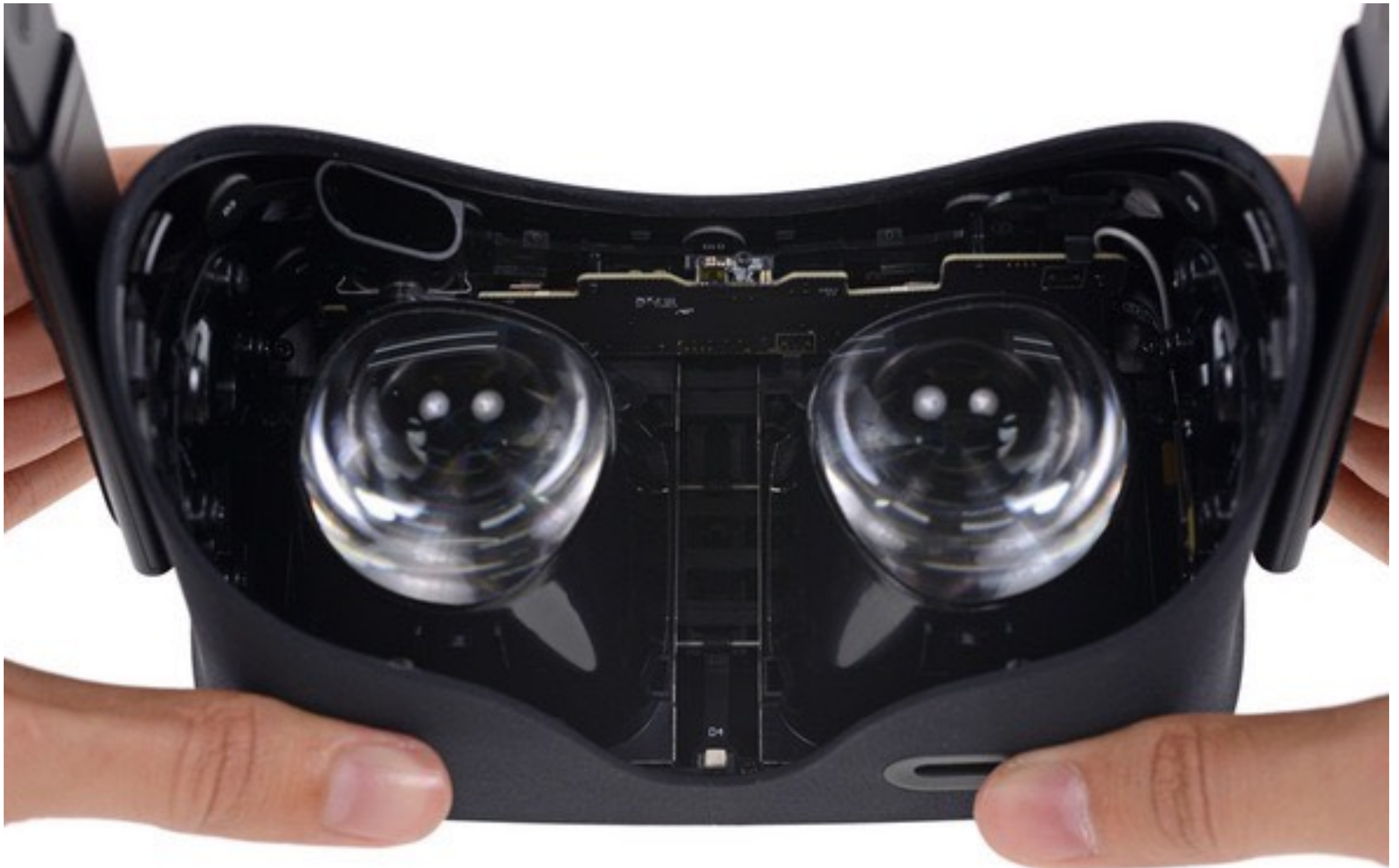
Intra-ocular distance adjustment
