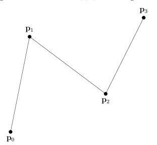
3. Show that the point with parameter *t* on the Bézier curve with control points  $\mathbf{p}_0$ ,  $\mathbf{p}_1$ ,  $\mathbf{p}_2$ ,  $\mathbf{p}_3$  is given by  $s^3\mathbf{p}_0 + 3s^2t\mathbf{p}_1 + 3st^2\mathbf{p}_2 + t^3\mathbf{p}_3$ , where s = 1 - t. (Hint: apply de Casteljau's algorithm algebraically to the control points. With this setup, linear interpolation between two points  $\mathbf{q}_0$  and  $\mathbf{q}_1$  looks like  $s\mathbf{q}_0 + t\mathbf{q}_1$ .)
