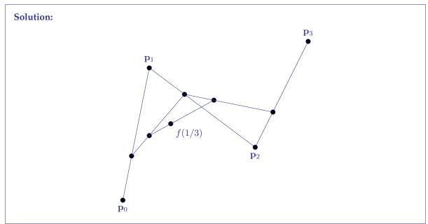
3. Show that the point with parameter t on the Bézier curve with control points  $\mathbf{p}_0$ ,  $\mathbf{p}_1$ ,  $\mathbf{p}_2$ ,  $\mathbf{p}_3$  is given by  $s^3\mathbf{p}_0+3s^2t\mathbf{p}_1+3st^2\mathbf{p}_2+t^3\mathbf{p}_3$ , where s=1-t. (Hint: apply de Casteljau's algorithm algebraically to the control points. With this setup, linear interpolation between two points  $\mathbf{q}_0$  and  $\mathbf{q}_1$  looks like  $s\mathbf{q}_0+t\mathbf{q}_1$ .)
