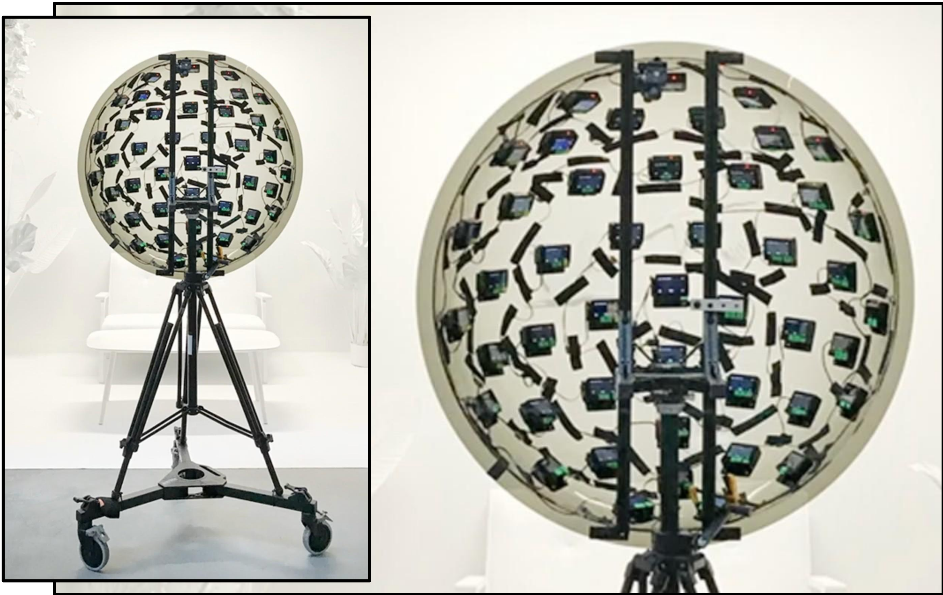
Google 6 DOF Light Field Camera. Broxton et al. 2019.
